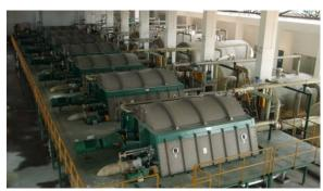
Together with GL&V, Microfusion assisted in the implementation of the GL&V DualC<sup>TM</sup> cooking process at the Chongqing mill. The DualC<sup>TM</sup> cooking process combines two-stage black liquor impregnation with a carefully controlled alkali and temperature profile specifically derived for bamboo cooking for optimal issue strength and properties. The cooking and washing process is completely automated and optimized using ABB 800xA DCS.
